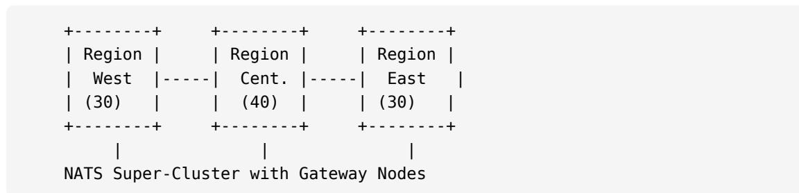
At national scale, NATS super-clusters provide inter-region communication with gateway nodes handling cross-region routing. Each region operates as an independent NATS cluster. Gateway nodes selectively bridge subjects between regions. The architecture scales horizontally – adding a new region is adding a new NATS cluster and configuring gateway connections.
