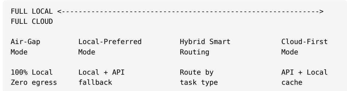
Each mode is a configuration of the same codebase. The Bike4Mind application binary is identical across all four modes. What changes is the set of adapters that are activated, the egress policy that is enforced, and the routing rules that determine where inference requests are sent.
